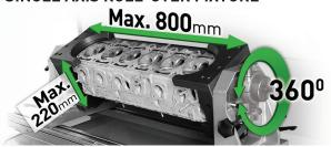
• Cylinder head clamping system that combined a side clamps for cylinder head, used for different angles with a universal mechanical fixture and rotatable adjustable 360° also for simple and combined angles.
